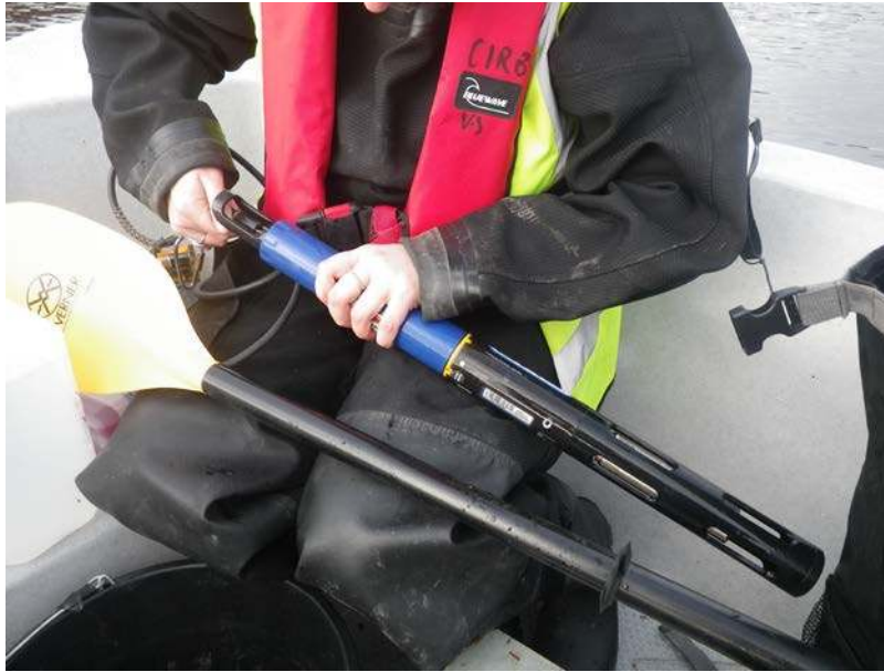
Figure 7: The multi-parameter sonde
