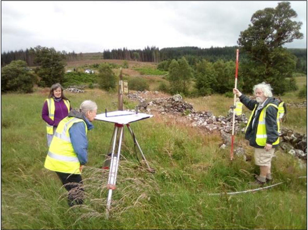
Plane Table Survey at Polmaddy deserted settlement (July 2019)
