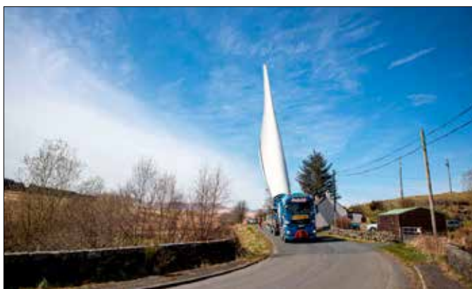
An elevated blade travelling along the B729 towards to site
