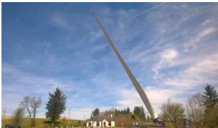
Photograph submitted by Rita Fairgrieve of a wind turbine blade being lifted to make it round a corner on the B729 next to her house, Old Burnfoot Cottage.
